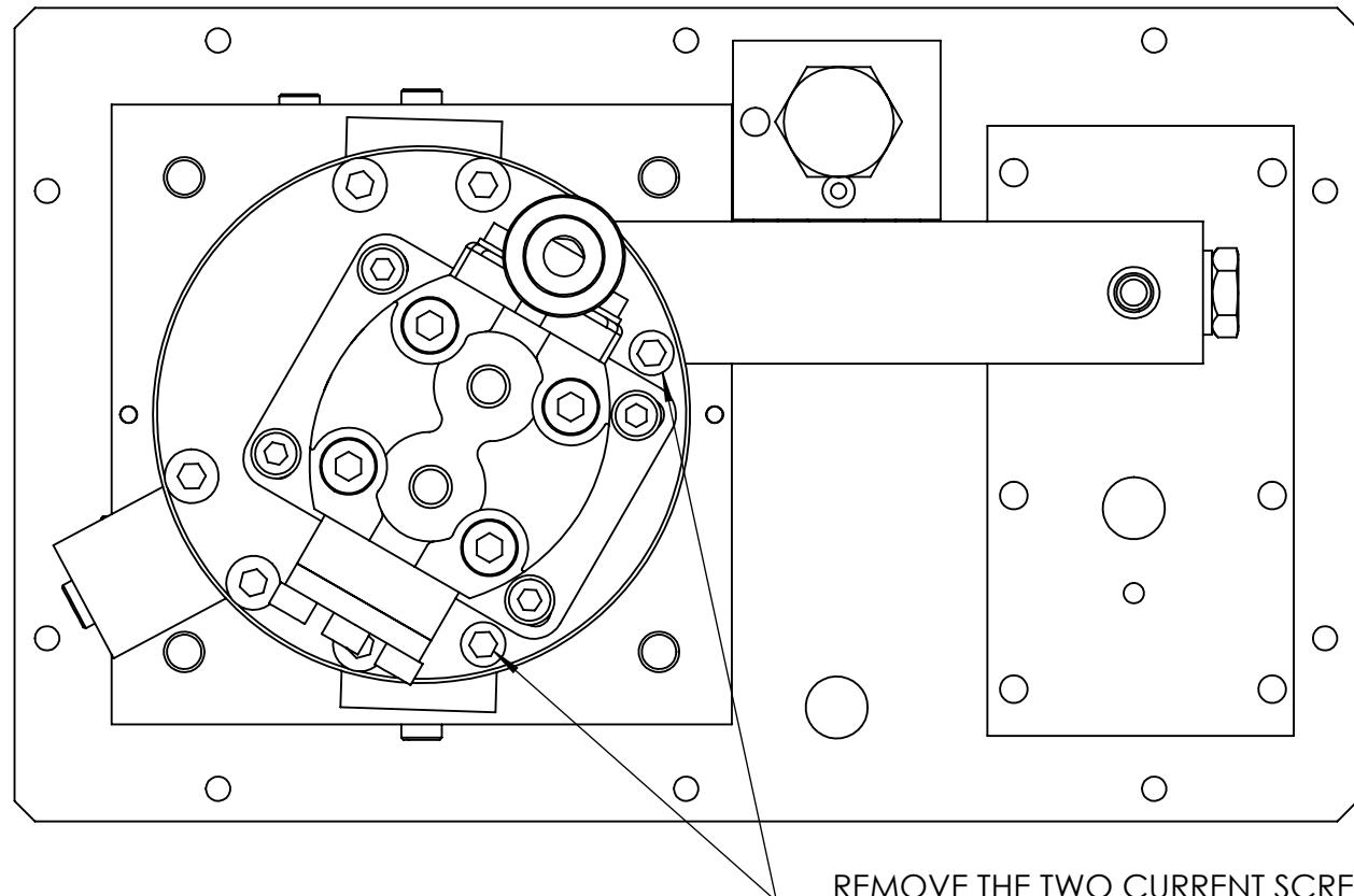
REMOVE THE TWO CURRENT SCREWS FROM THESE TWO
